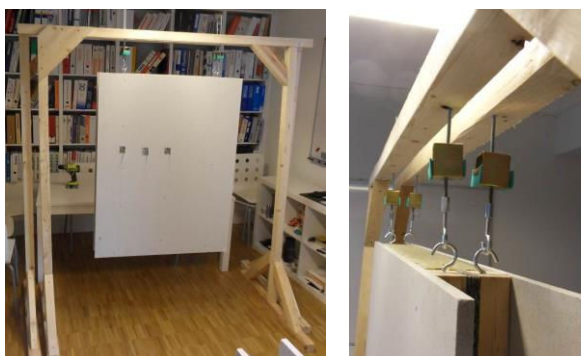
Figure 1. Experimental setup, sample suspended with isolated hangers).
