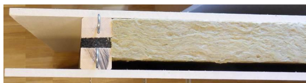
Figure 2. Sample NBW2 for non-bearing wall (100 mm including 20 mm rubber).
