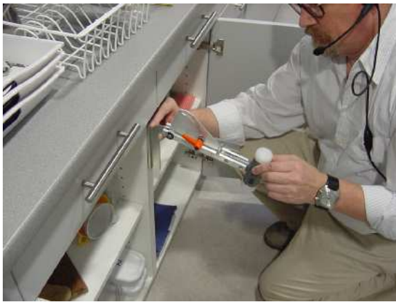
Figure 2: Horizontal measurement with the pendulous hammer.
