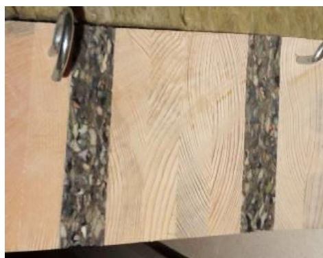
Figure 3. Sample BW4 for bearing wall (200 mm including 2x20 mm composite foam).
